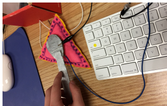
Figure 2: Non-wearable controller: spoon taps the cake, which completes the circuit.
