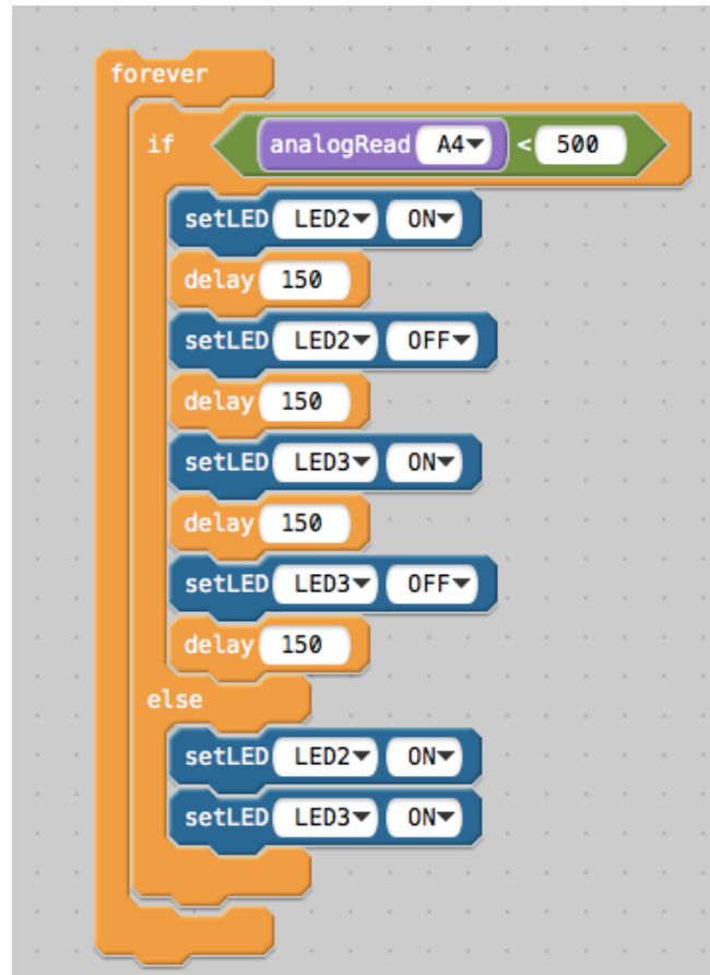
Figure 4: Code for Jason’s completed project showing rapid blinking when patches are touched.
