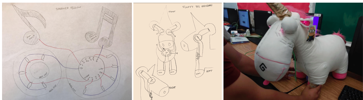
Figure 2. Two Circuit Diagram DebugIts, which included circuit drawings (left, middle) with mistakes such as short circuits, ungrounded LEDs, and sensor patches connected to the wrong microcontroller pins. (right) Shown here is the past project of an actual students, which inspired our circuit DebugIt (middle).
