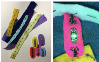
Figure 2: Reconstruction Kit for E-Textiles. Functional LilyPad circuit (top); modular felt strips with metallic thread (bottom left) and hooked LEDs (bottom right) to bypass sewing
