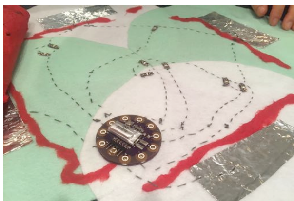
Figure 2: Prototype of Collaborative e-Textile Centerpiece (top) and backside with stitched circuit design and LilyPad Arduino (bottom).
