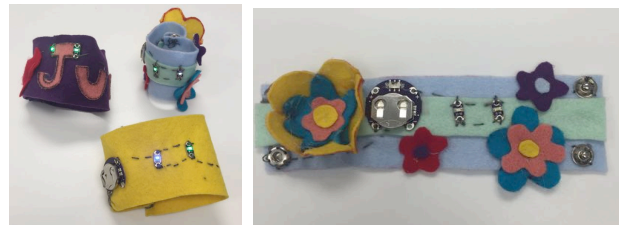
Figure 1: Examples of e-Textile Bracelet with snaps and LED (left) and the back of bracelet with battery holder (right).
