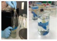
**B. BioSensor** construction using bacteria as detector: (left) Putting the transformed bacteria into the dialysis bag; (right) The completed sensor contraption. Source: Kafai et al., 2017.
