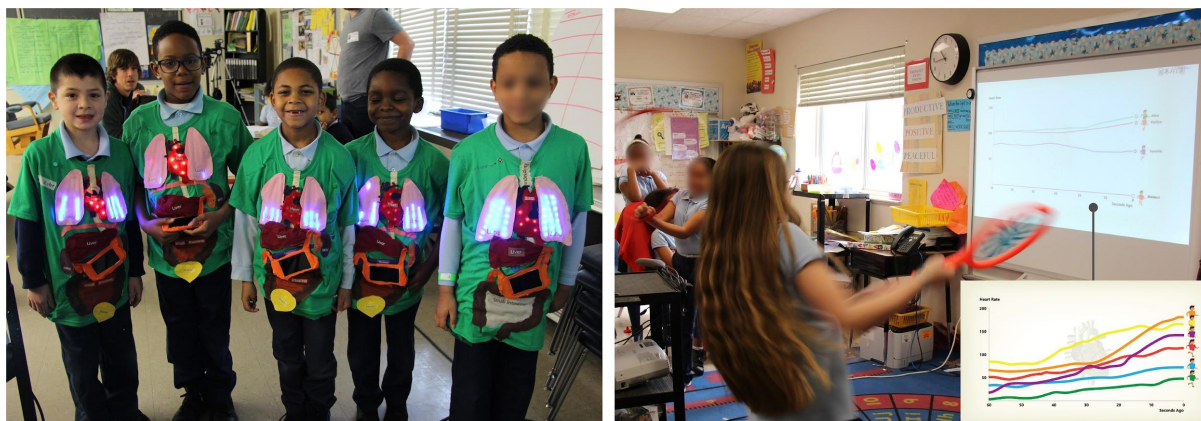
Figure 3. BodyVis (left) and SharedPhys (right) are two LPSV tools that visualize wearers' live body-data on an electronic textile (e-textile) shirt and a large-screen display respectively.
