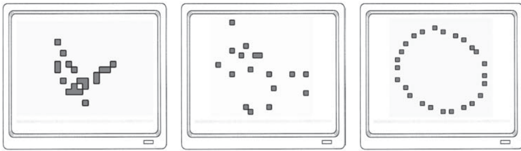
Figure 3.2. These screen shots show a new way to create a circle with StarLogo. No single turtle draws the circle. Rather, the turtles arrange themselves into a circle, based on their interactions with one another. Each turtle follows two simple rules: (1) it tries to keep a certain distance from each of its two “neighbors,” and (2) it gently “repels” the group as a whole, trying to move away from the other turtles. With these two rules, the turtles arrange themselves into a circle. (Adapted with permission from the StarLogo Web site at http://education.mit.edu/starlogo/ .)
